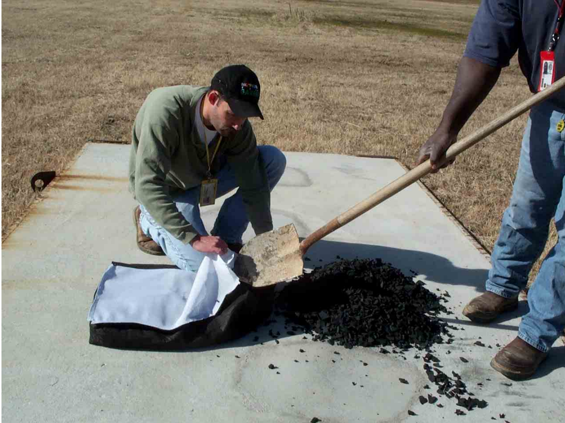
Figure 1. Filling Filter Elements Units at the Corps of Engineers Test Site. The white side of the filter unit is a nylon open mesh, the black fabric is a punch-woven nylon-polypropylene geofabric designed for soil drainage.
